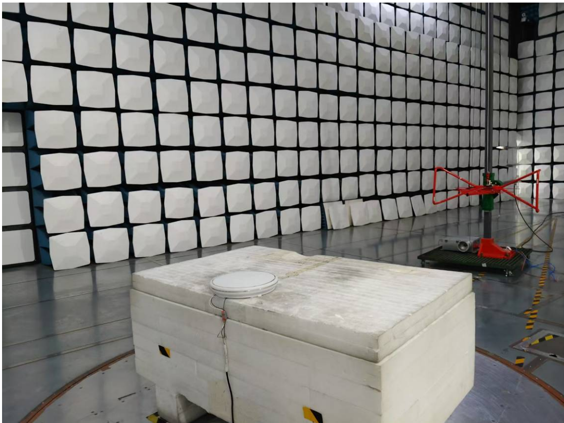
Radiated Emission 30MHz -1GHz Rear View
