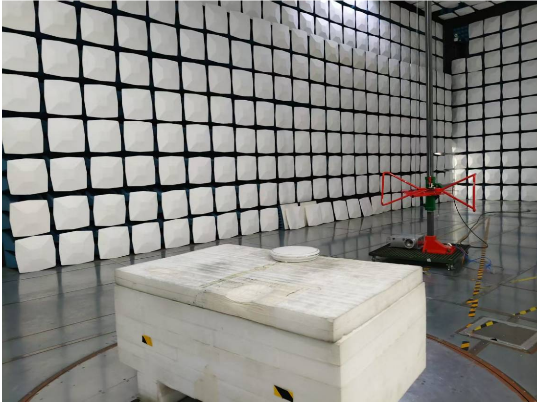
Radiated Emission 30MHz -1GHz Rear View
