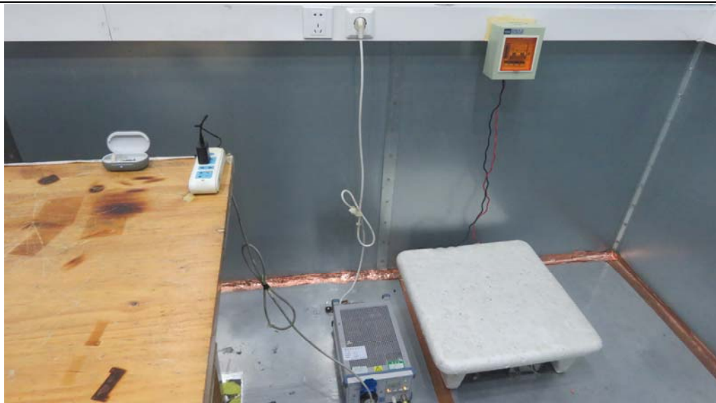
Picture 2: Conducted Emissions Test Setup
