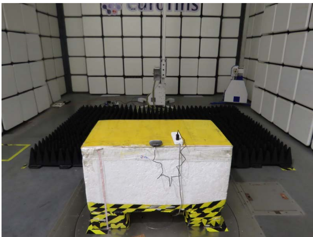
Picture 1: Radiated Emission Test Setup
