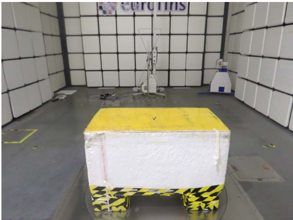
Picture 1 Radiated Emission Test Setup
