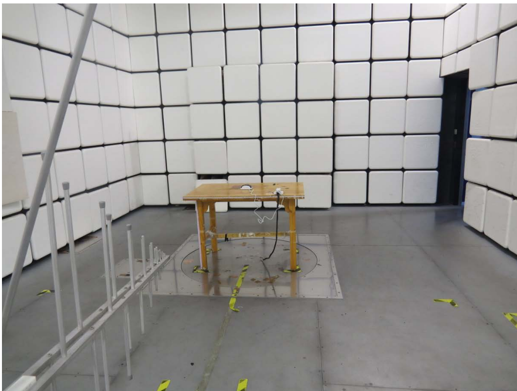
Picture 2 Radiated Emission Test Setup
