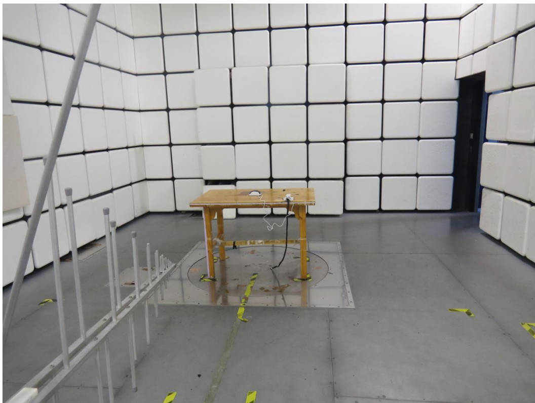
Picture 2 Radiated Emission Test Setup
