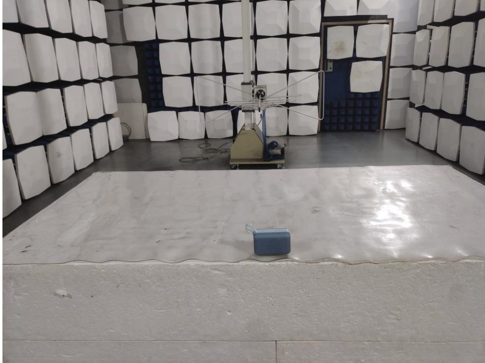
Radiated Emission Test Setup:
