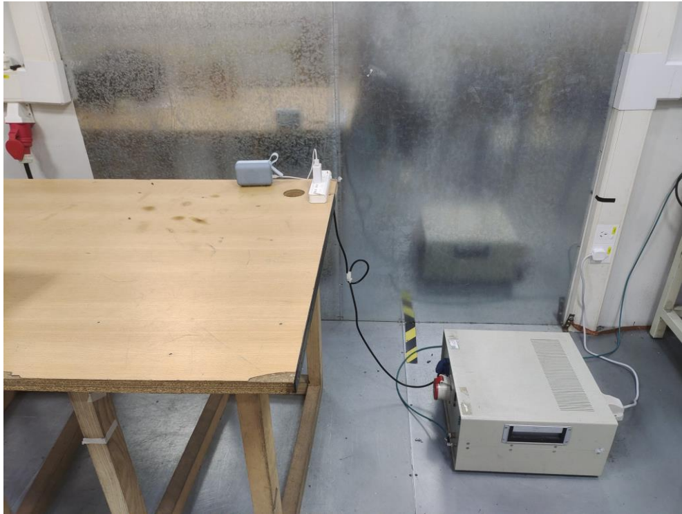
Conducted Emission Test Setup:
