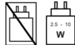
The power delivered by the charger must be between min 2.5 Watts required by the radio equipment, and max 10 Watts in order to achieve the maximum charging speed.
