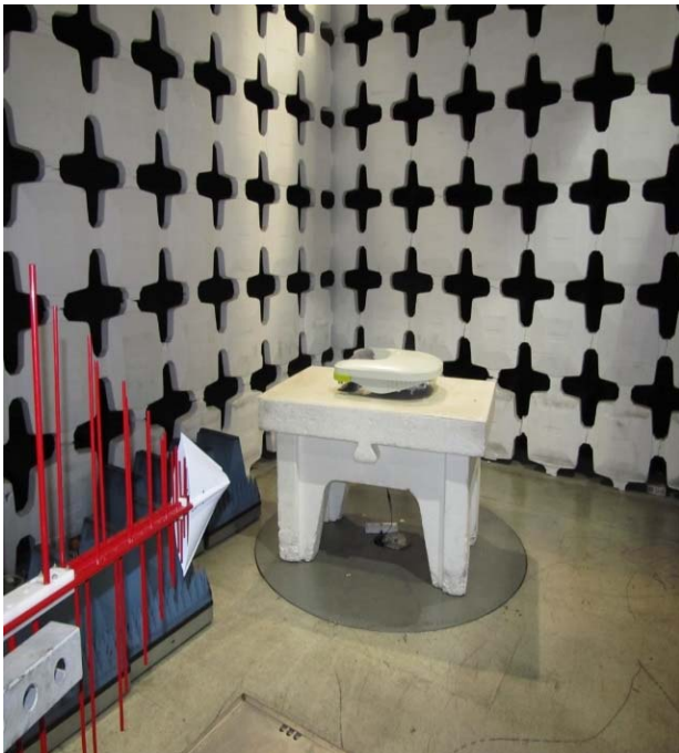
Radiated emissions test setup with Biconilog antenna.
