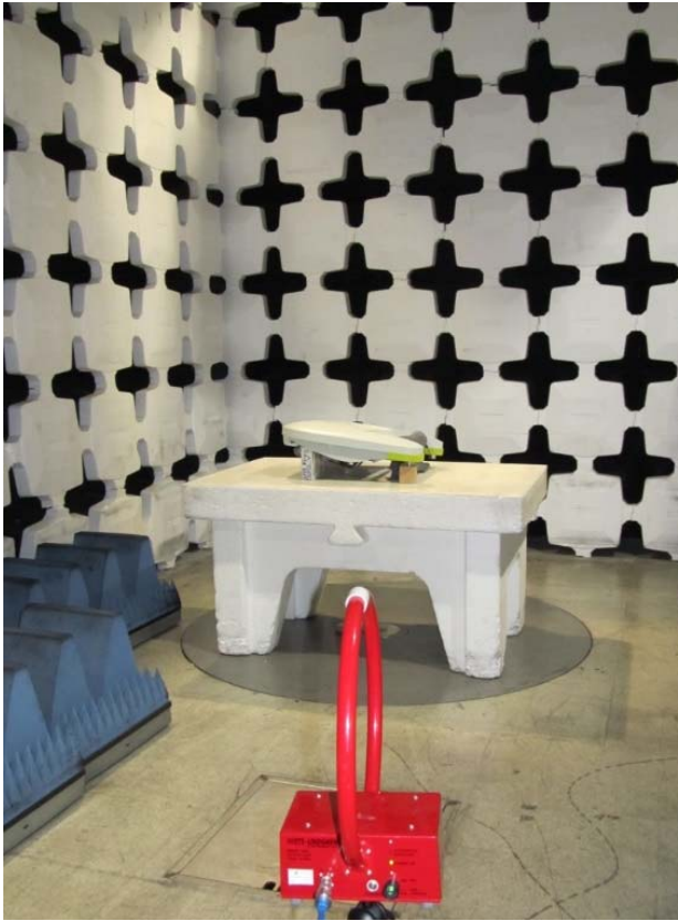
Radiated emissions test setup with Loop antenna.
