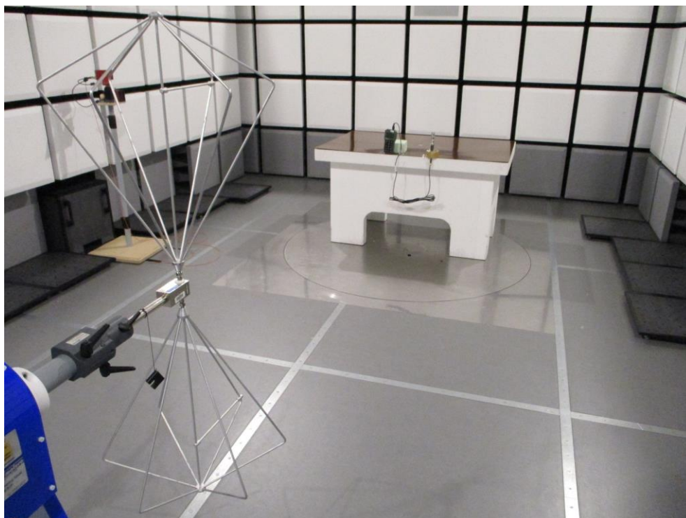
Figure 2: Radiated emission test from 30 MHz to 200 MHz
