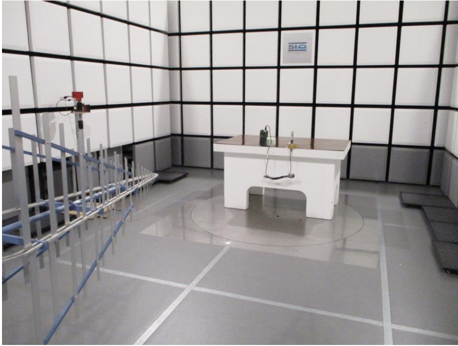
Figure 3: Radiated emission test from 200 MHz to 1 GHz
