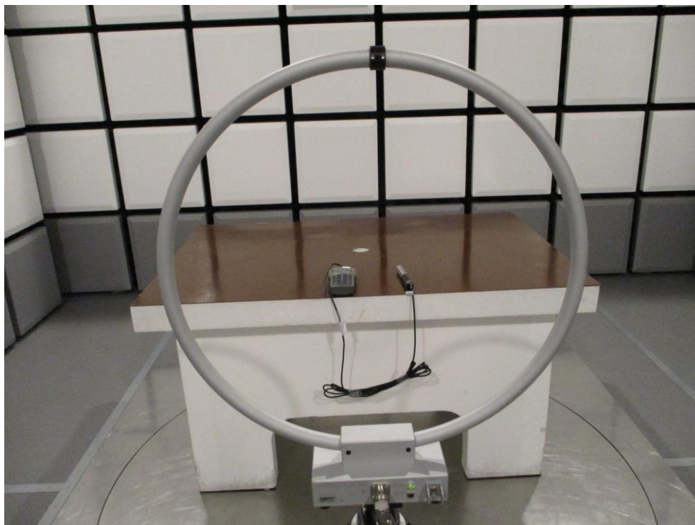
Figure 1: Radiated emission test from 9 kHz to 30 MHz
