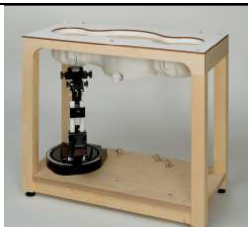
Fig. 8.7 Photo of SAM Twin Phantom
