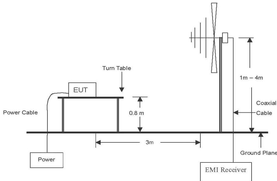
The diagram below shows the test setup that is utilized to make the measurements for emission from 1 GHz to the tenth harmonic of the highest fundamental frequency or to 40 GHz emissions, whichever is lower.
