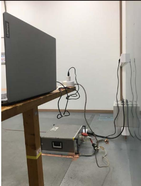
**RADIATED EMISSION TEST****-. 900 MHz(LoRa)**
