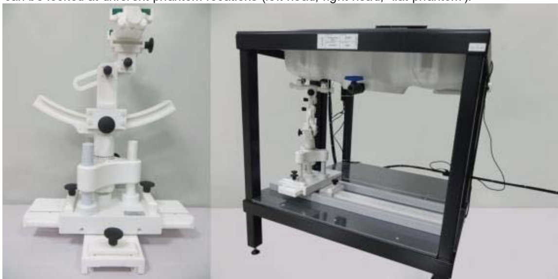
Device holder supplied by SATIMO
