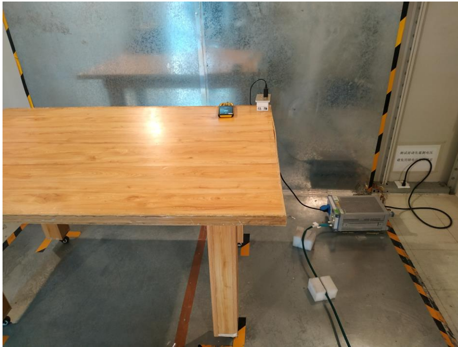
Conducted Emissions (Side View)
