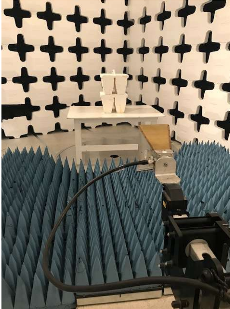
Figure 6. Radiated Emissions Test Configuration (Above 1 GHz)
