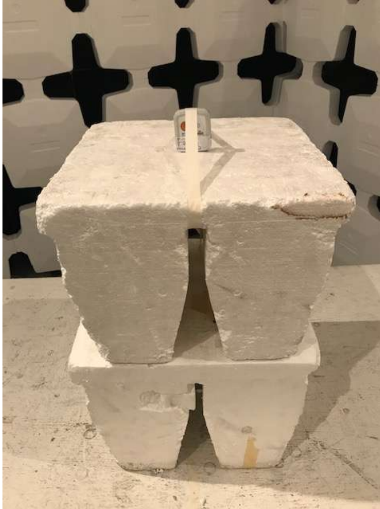
Figure 5. EUT Raised to 1.5 m
