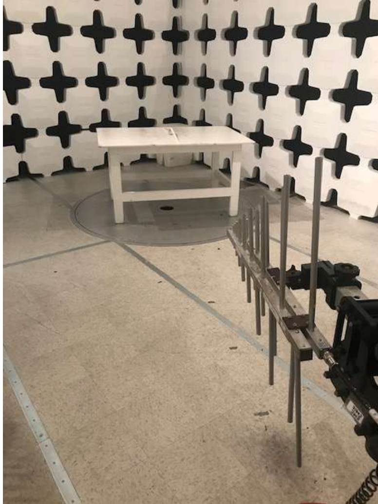
Figure 4. Radiated Emissions Test Configuration (200 MHz to 1 GHz)
