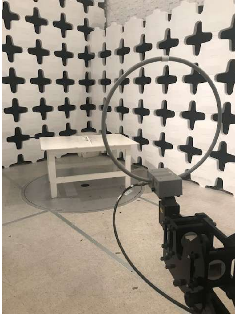
Figure 2. Radiated Emissions Test Configuration (Below 30 MHz)
