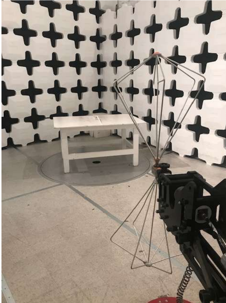
Figure 3. Radiated Emissions Test Configuration (30-200 MHz)
