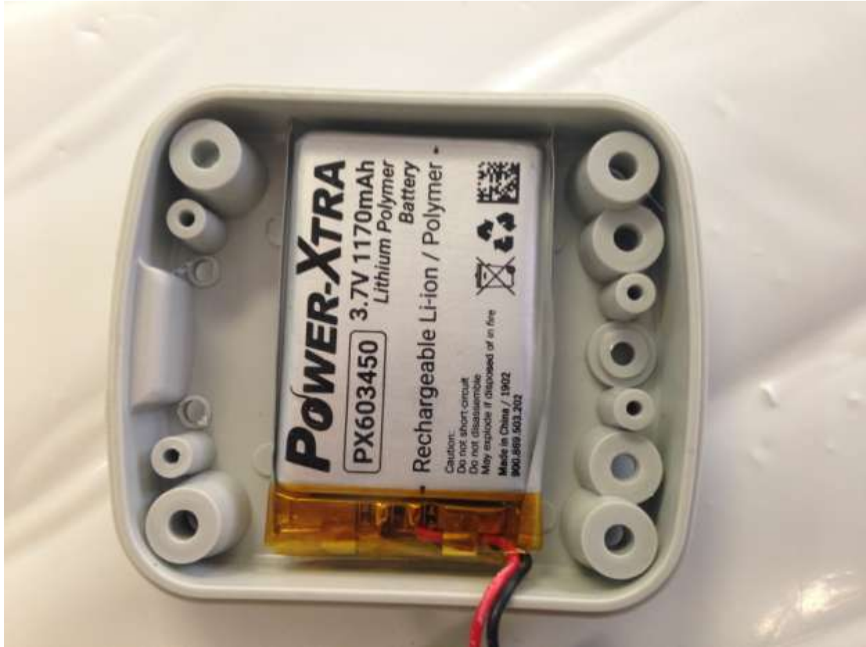
Figure 5. Back Cover with Battery Pack Exposed
