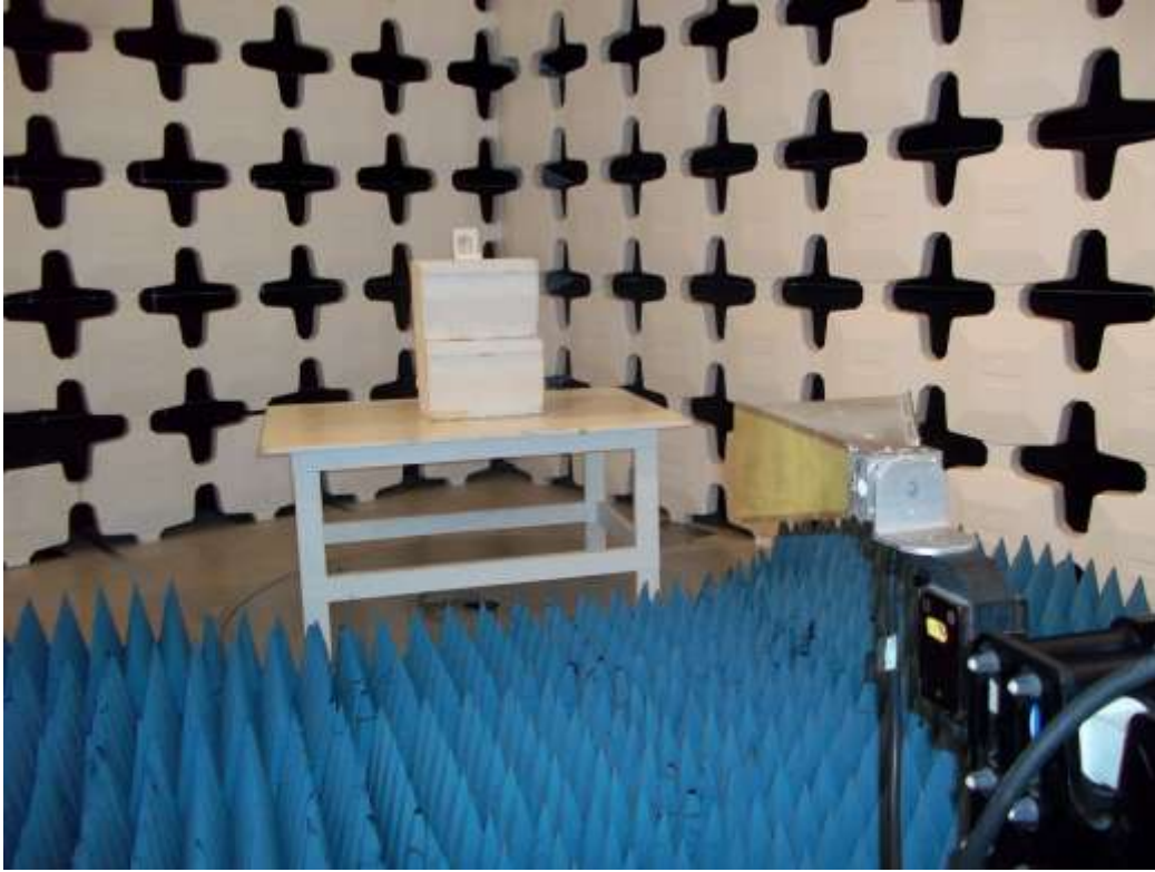
Figure 4. Radiated Emissions Test Configuration (Above 1 GHz)
