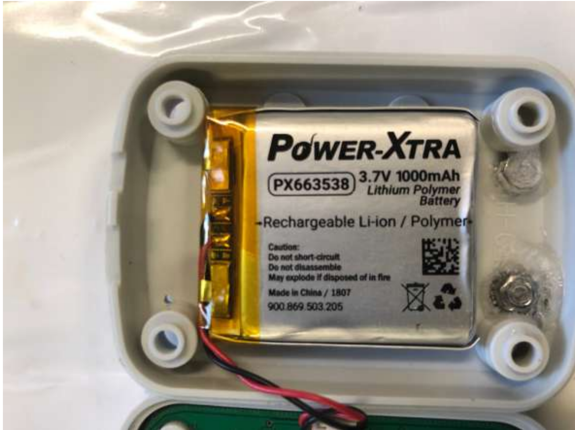
Figure 8. Seated Battery Pack
