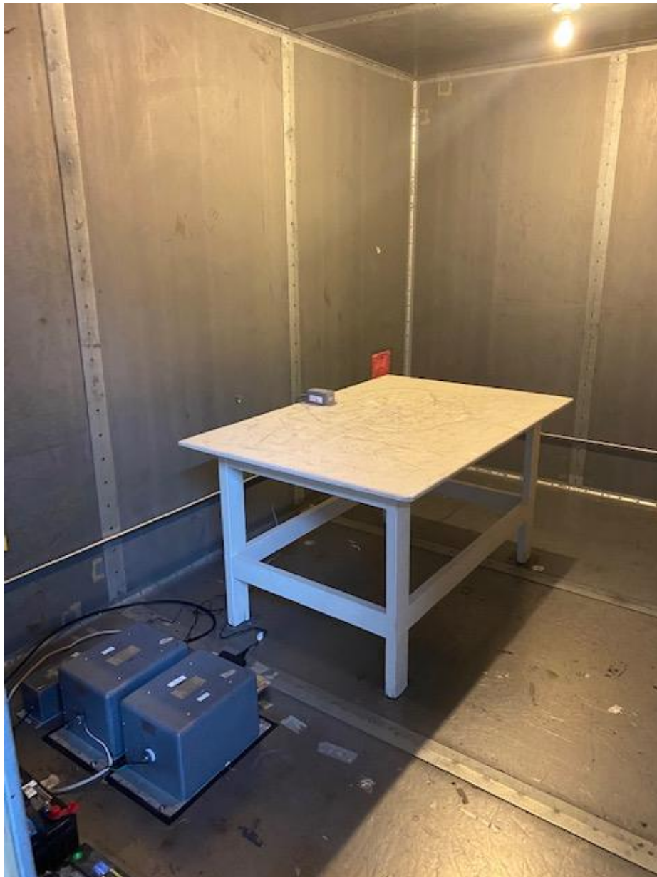
Figure 6. Power Line Conducted Emissions Test Configuration
