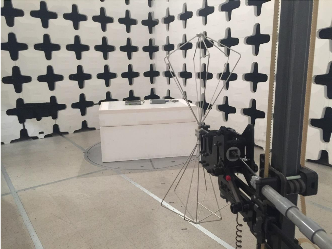
Figure 3. Radiated Emissions Test Configuration (30-200 MHz)
