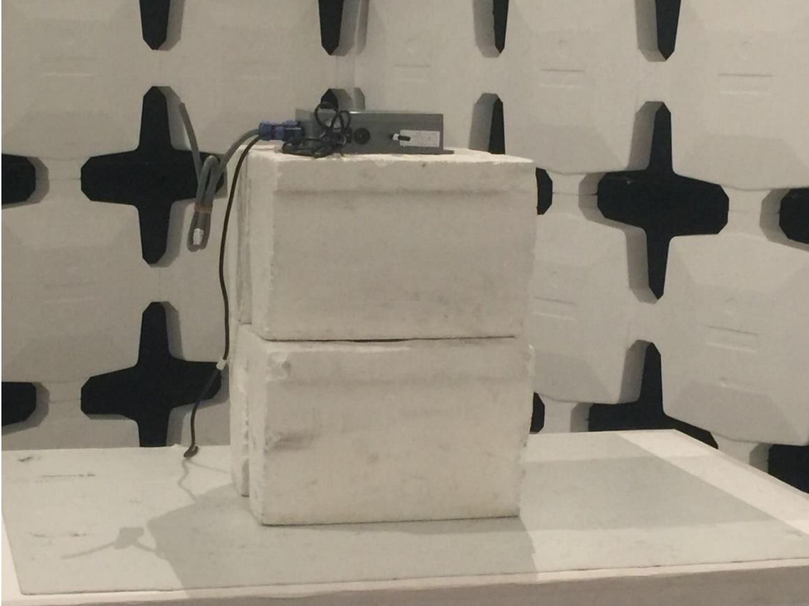
Figure 5. EUT Raised to 1.5 m
