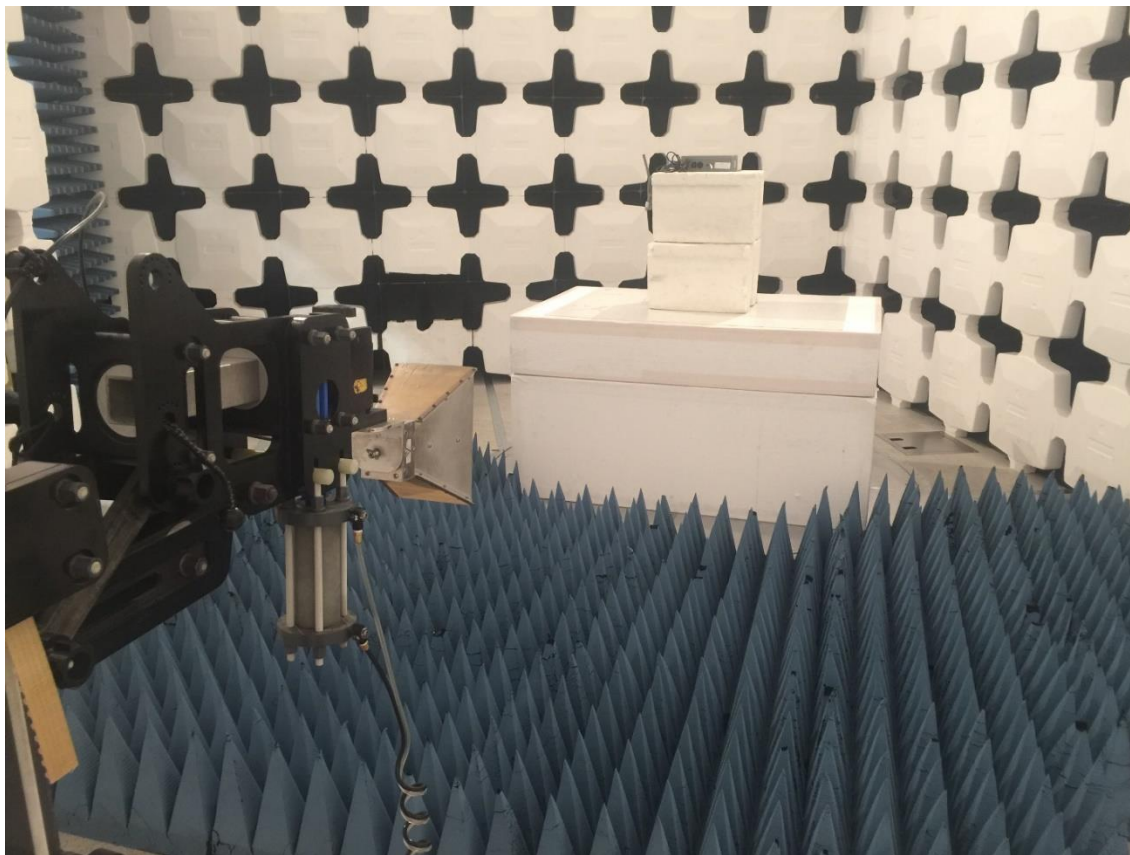
Figure 6. Radiated Emissions Test Configuration (Above 1 GHz)
