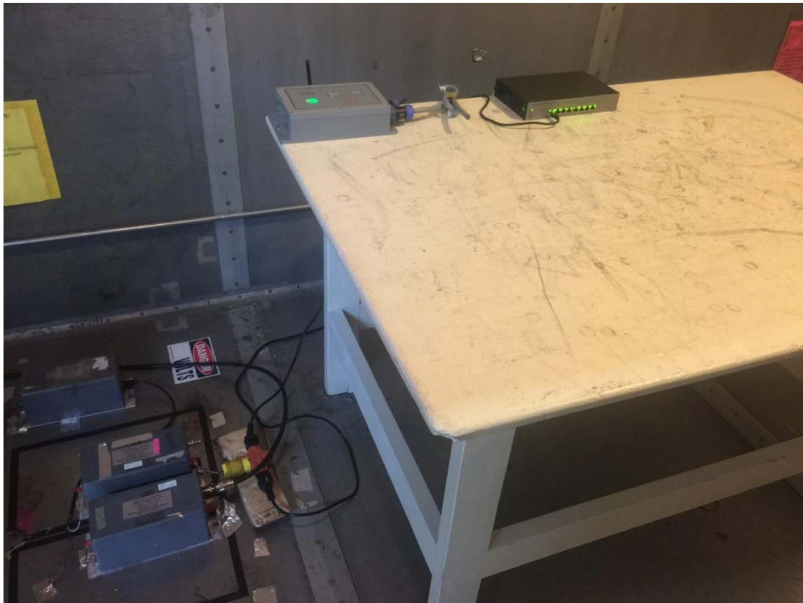
Figure 7. Power Line Conducted Emissions Test Configuration
