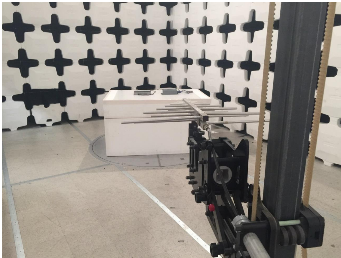
Figure 4. Radiated Emissions Test Configuration (200 MHz to 1 GHz)
