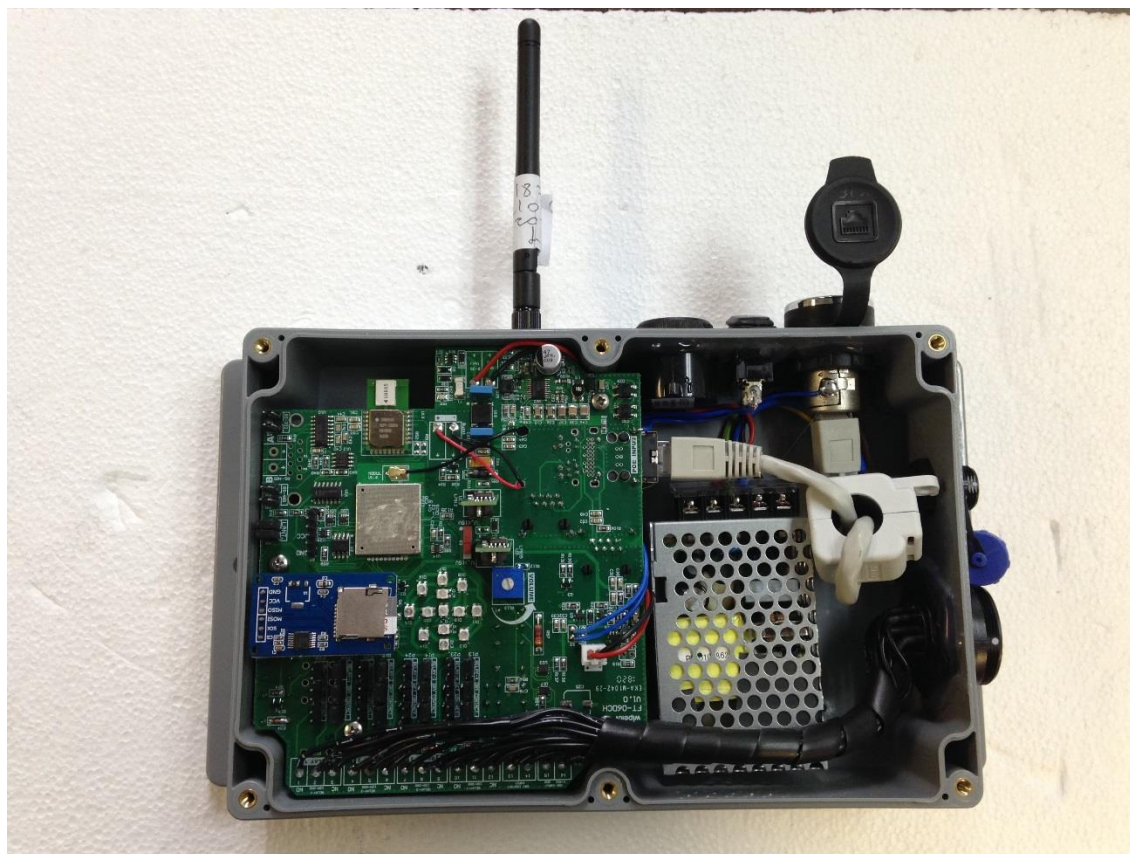
Figure 2. EUT, FT-06DCH-POE-IO, Internal Electronics
