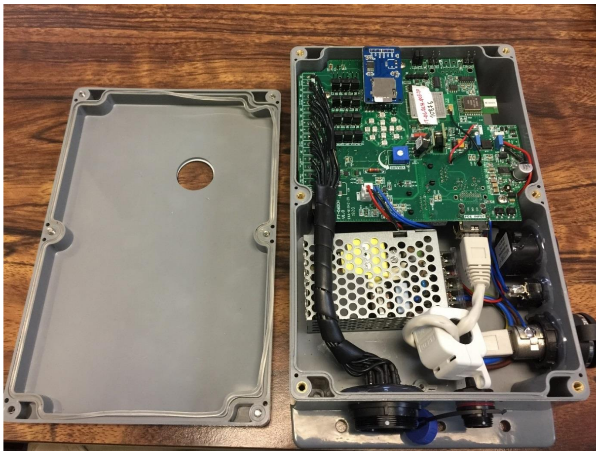
Figure 1. FT-06DCH-POE-IO, Cover Open
