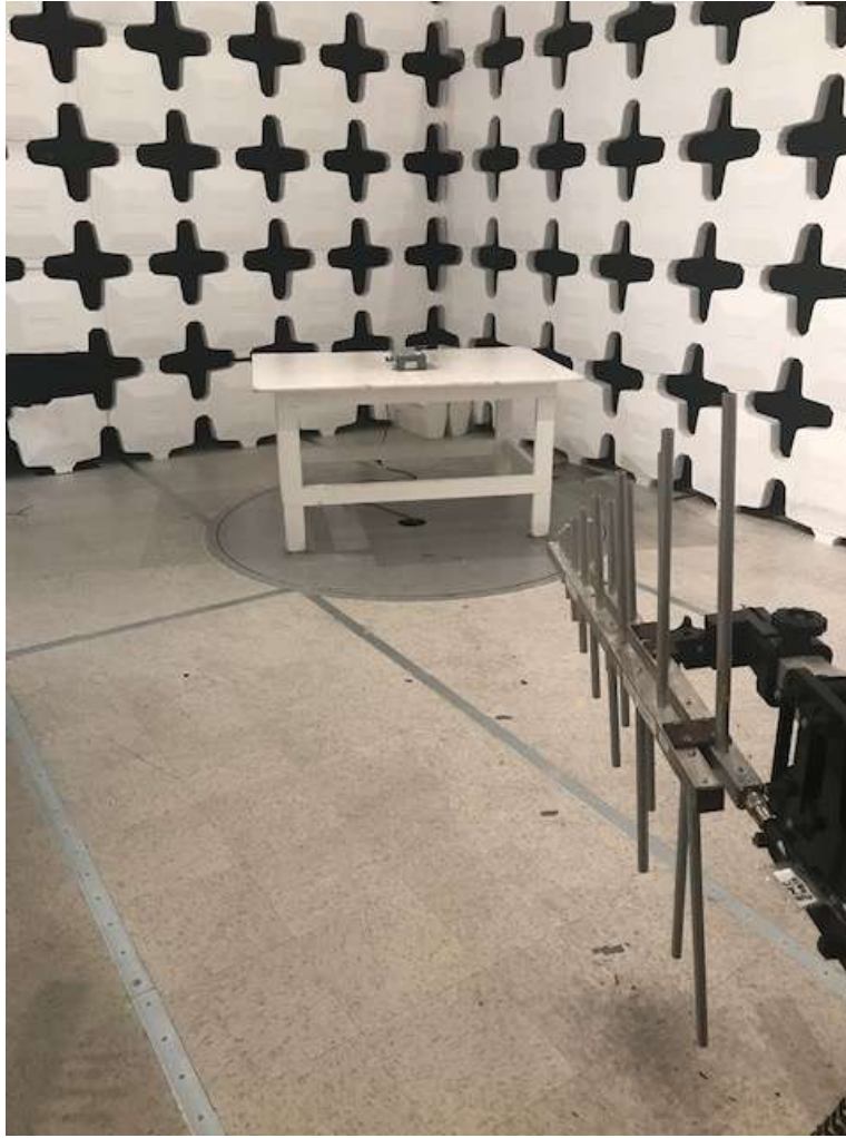
Figure 4. Radiated Emissions Test Configuration (200 MHz to 1 GHz)
