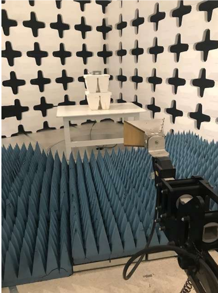
Figure 6. Radiated Emissions Test Configuration (Above 1 GHz)
