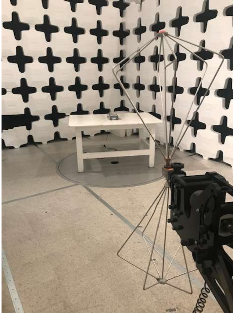
Figure 3. Radiated Emissions Test Configuration (30-200 MHz)
