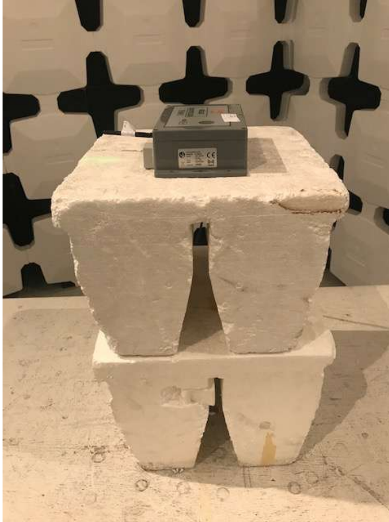
Figure 5. EUT Raised to 1.5 m
