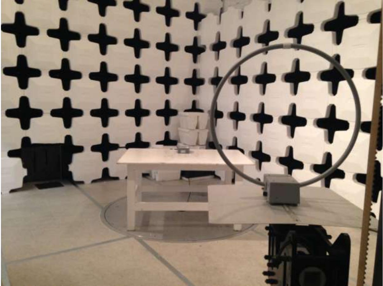
Figure 2. Radiated Emissions Test Configuration (Below 30 MHz)
