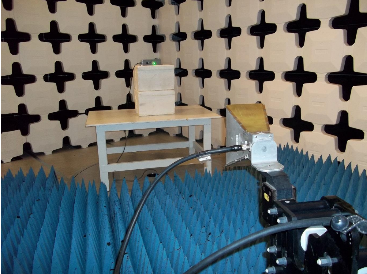
Figure 4. Radiated Emissions Test Configuration (Above 1 GHz)
