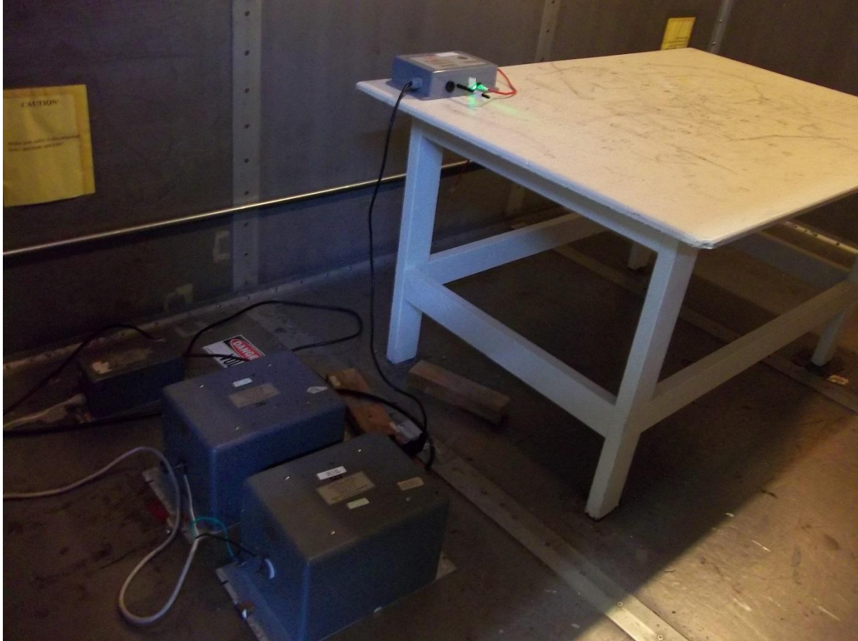
Figure 5. Power Line Conducted Emissions
