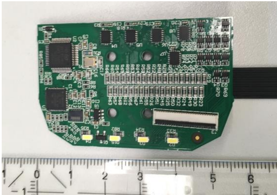
Display Board Top Side View
