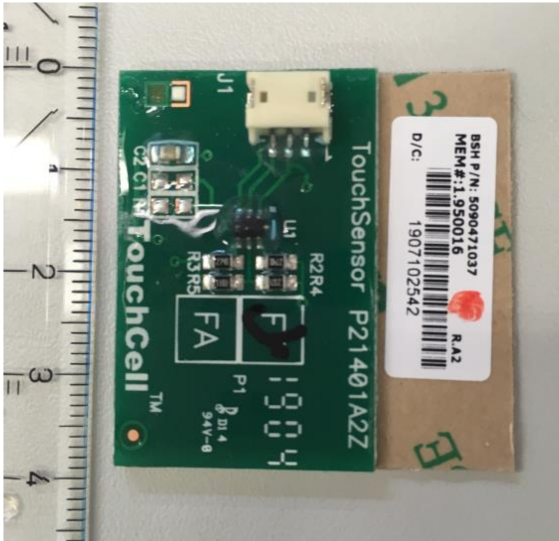
Water Level Sensor Top Side View
