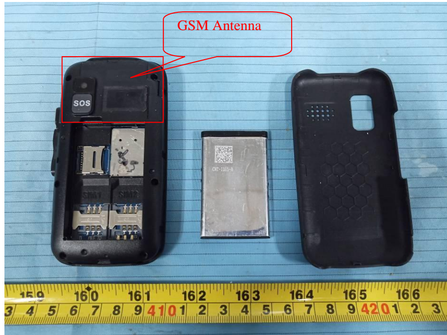
EUT – Cover off View 1
