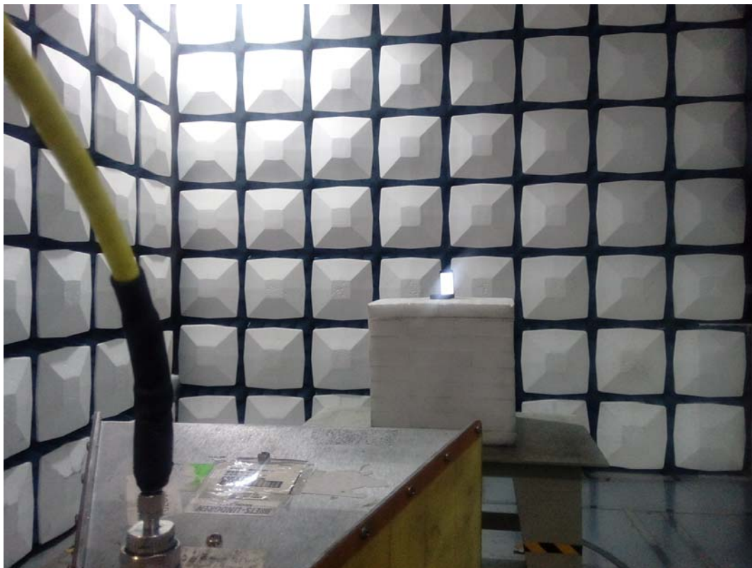
Radiated Emission Above 1GHz View
