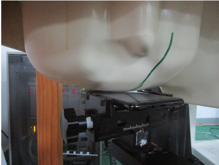
Head Right Check Setup Photo
