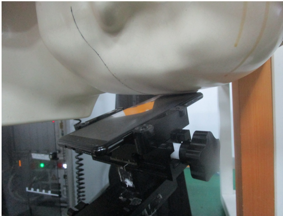
Head Left Tilt Setup Photo
