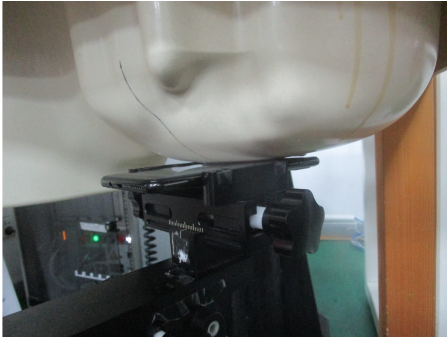
Head Left Cheek Setup Photo
