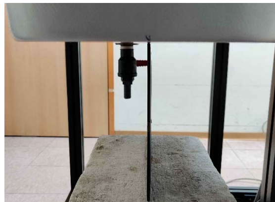
Fig.6 EUT Right side to flat phantom
