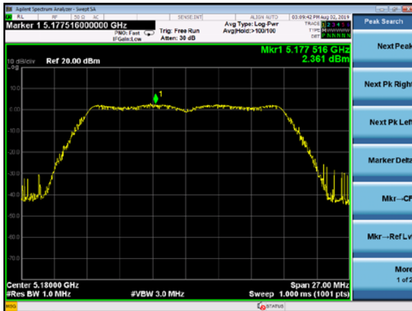
(802.11a) PSD plot on channel 36
