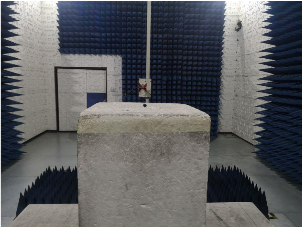
RADIATED EMISSION TEST SETUP ABOVE 1GHz
