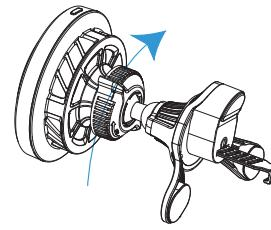
3. Turn the pulley to the left to adjust the hook to the longest.
