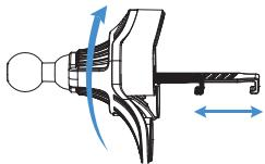
4. Rotate the pulley to the right to make the hooks to clamp the air vent blades.
