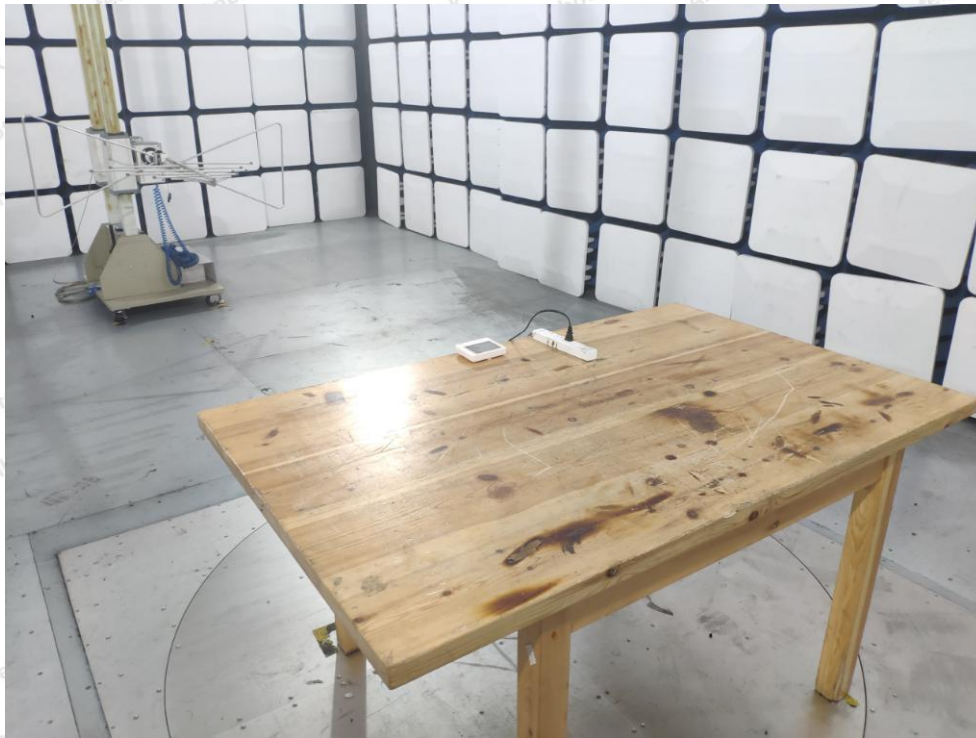
Photo of Radiation Emission Test
