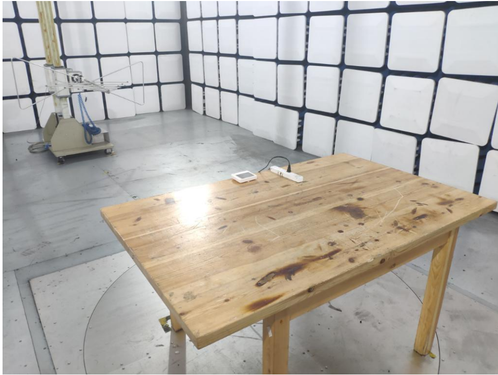
FCC ID: 2AUDN-STN855W Photo of Radiation Emission Test
