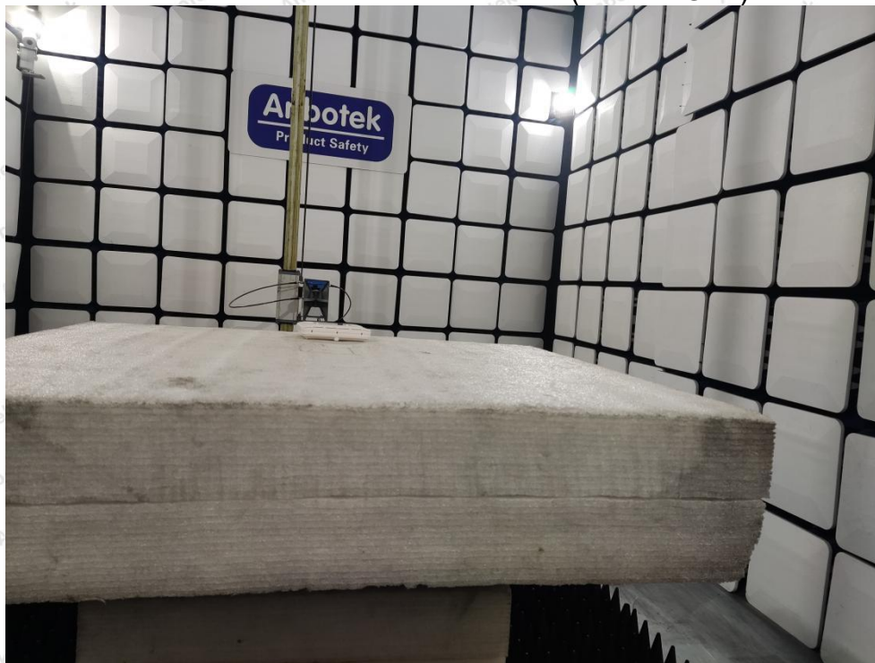
Photo of Radiation Emission Test (above 1GHz)
