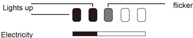
2. When the robot cleaner starts to work underwater, the indicator light is on, when the work is done, the indicator light all off.
