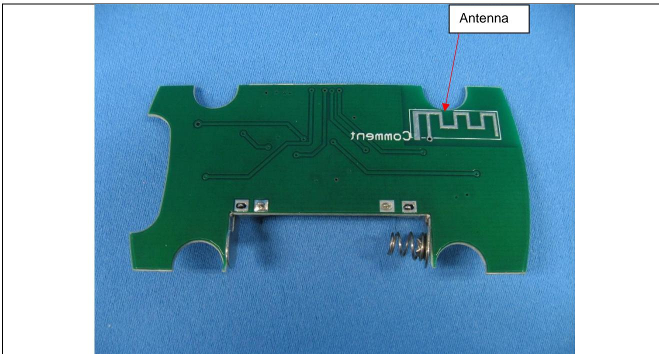
Details of: Battery view for remote control
