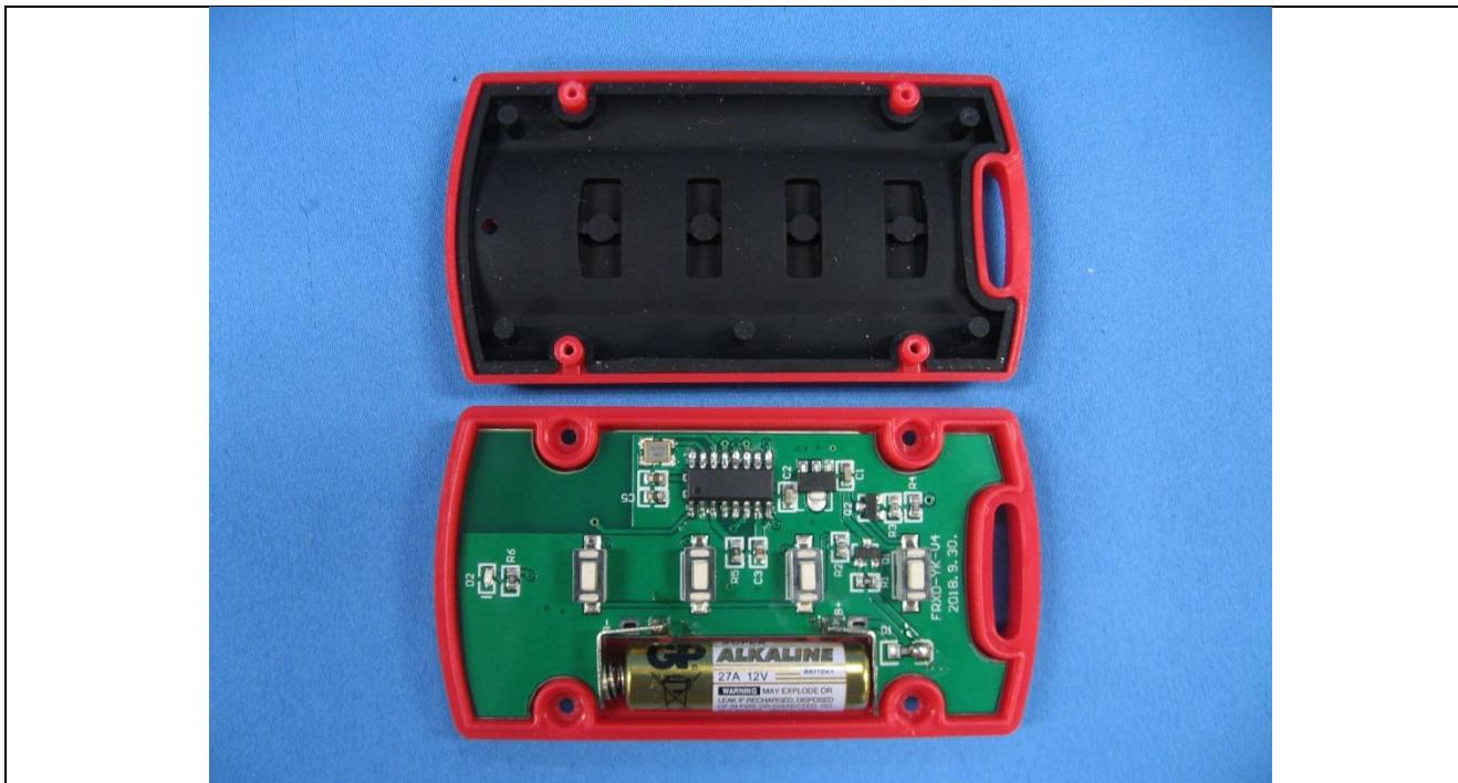
Details of: PCB view for remote control
