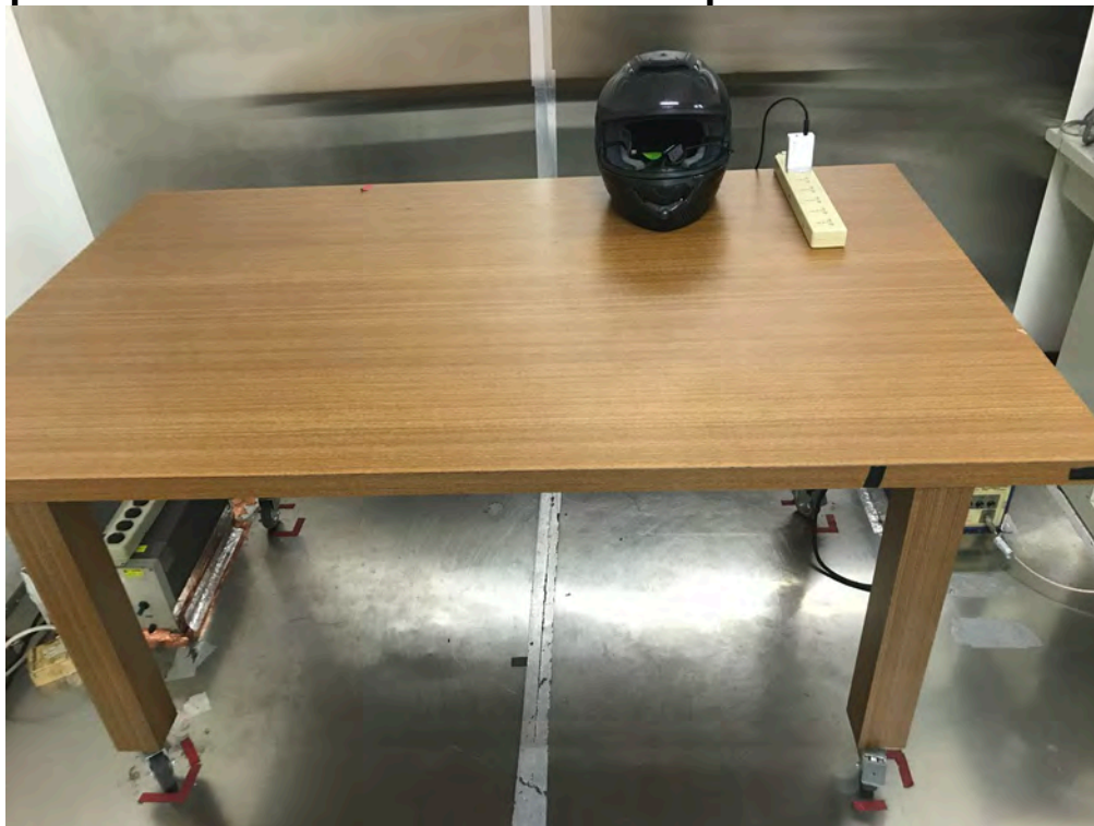
Photograph – Conducted Emission Test Setup
