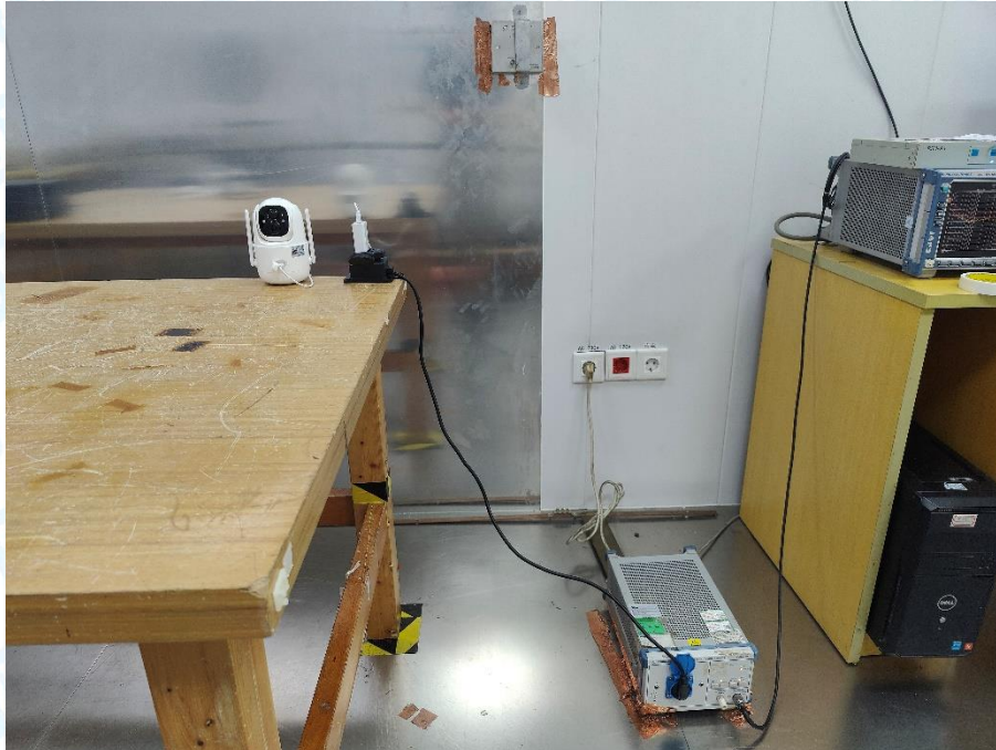
Photo of Setup for Radiated Emission (30MHz~1GHz)
