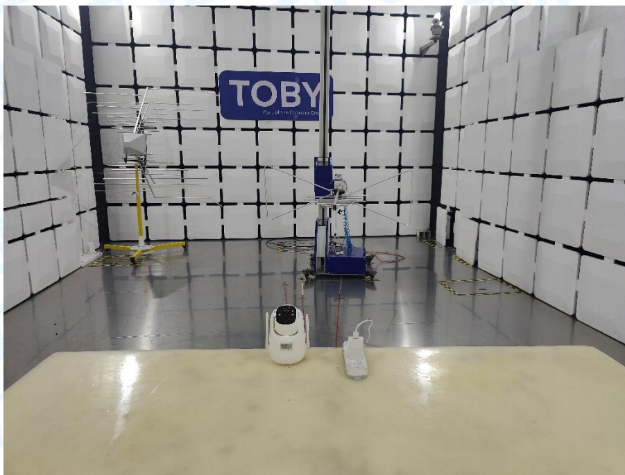
Photo of Setup for Radiated Emission (30MHz~1GHz)
