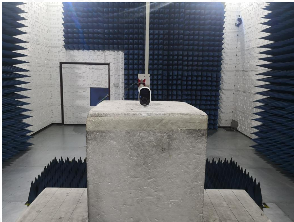
FCC RADIATED EMISSION TEST SETUP ABOVE 1GHZ
