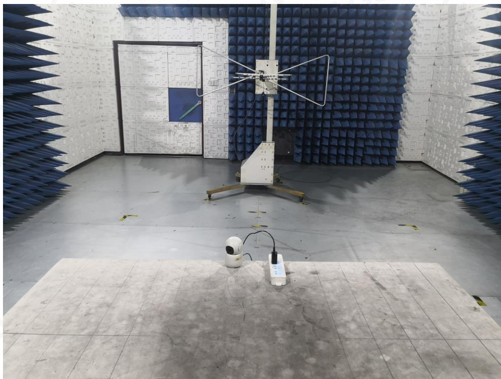
FCC RADIATED EMISSION TEST SETUP ABOVE 1GHZ
