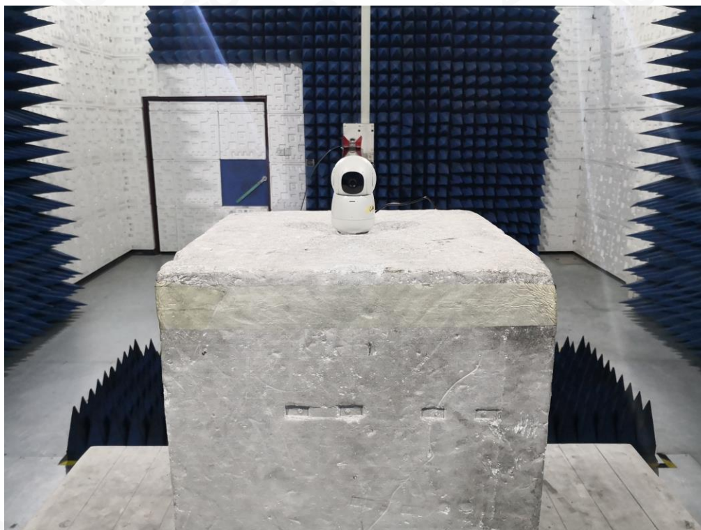
FCC RADIATED EMISSION TEST SETUP ABOVE 1GHZ
