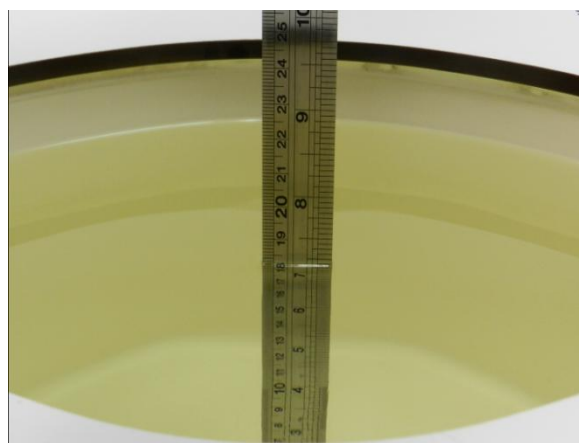
Fig 11.2 Photo of Liquid Height for Body SAR
