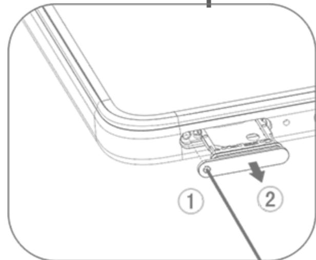
2. Place your nano-SIM card into the SIM 1 or SIM 2 holder in the direction of the arrow as shown in the illustration. Make sure to align the angled corner to the notch on the holder.
