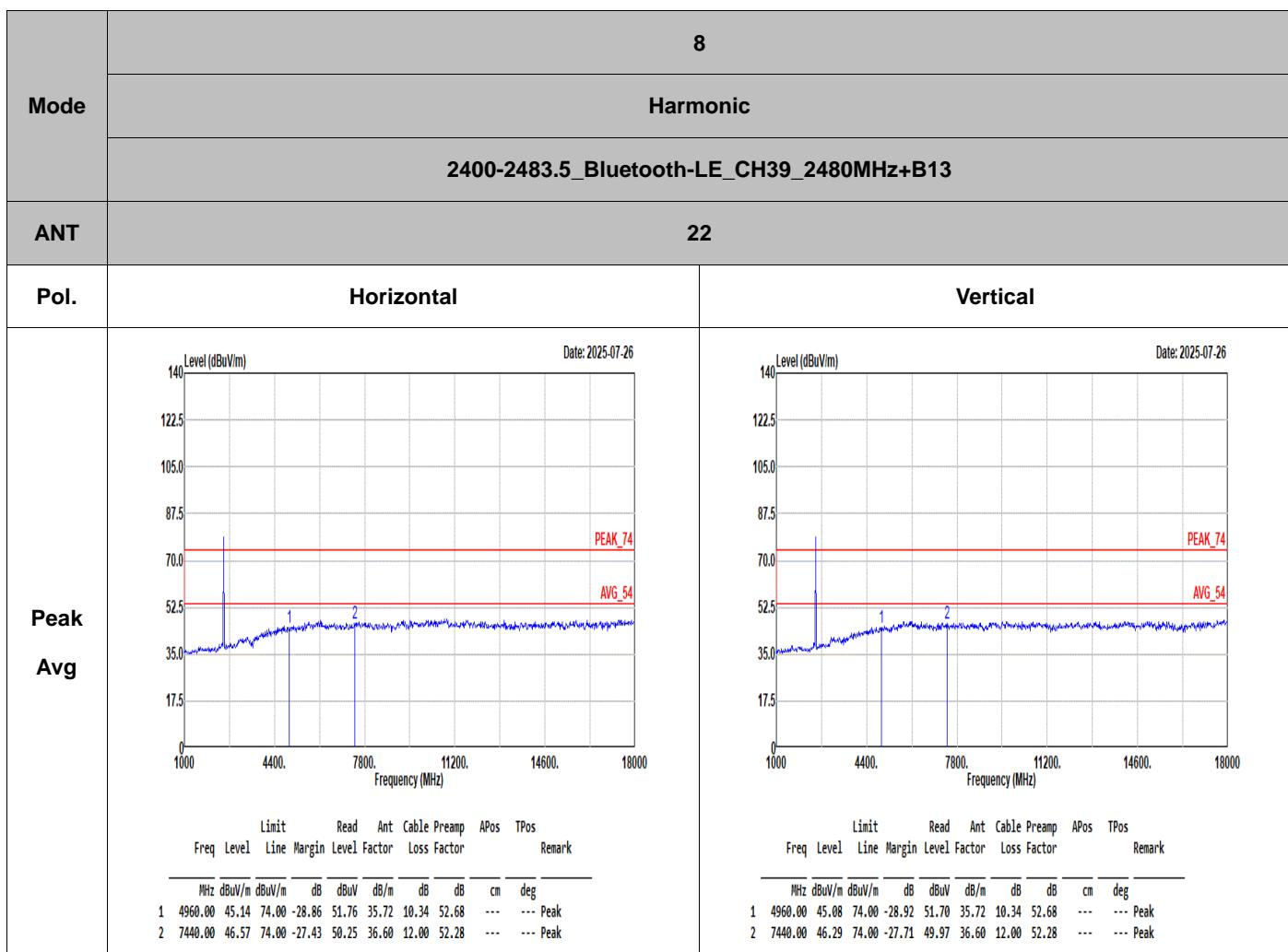
Note: For the frequency point over limit line is fundamental signal, which can be ignored.
