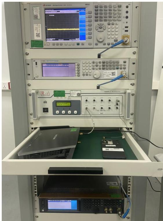
Remark: The setup for DFS Performed by SGS-CSTC Standards Technical Services Co., Ltd. Shenzhen Branch.
