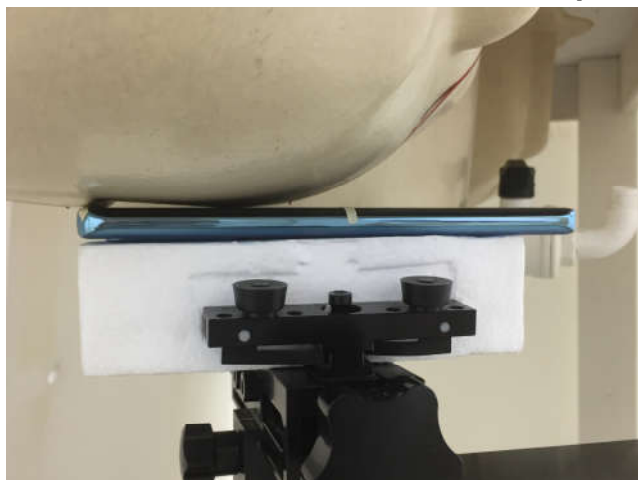
Right Cheek, Test Separation 0 mm
