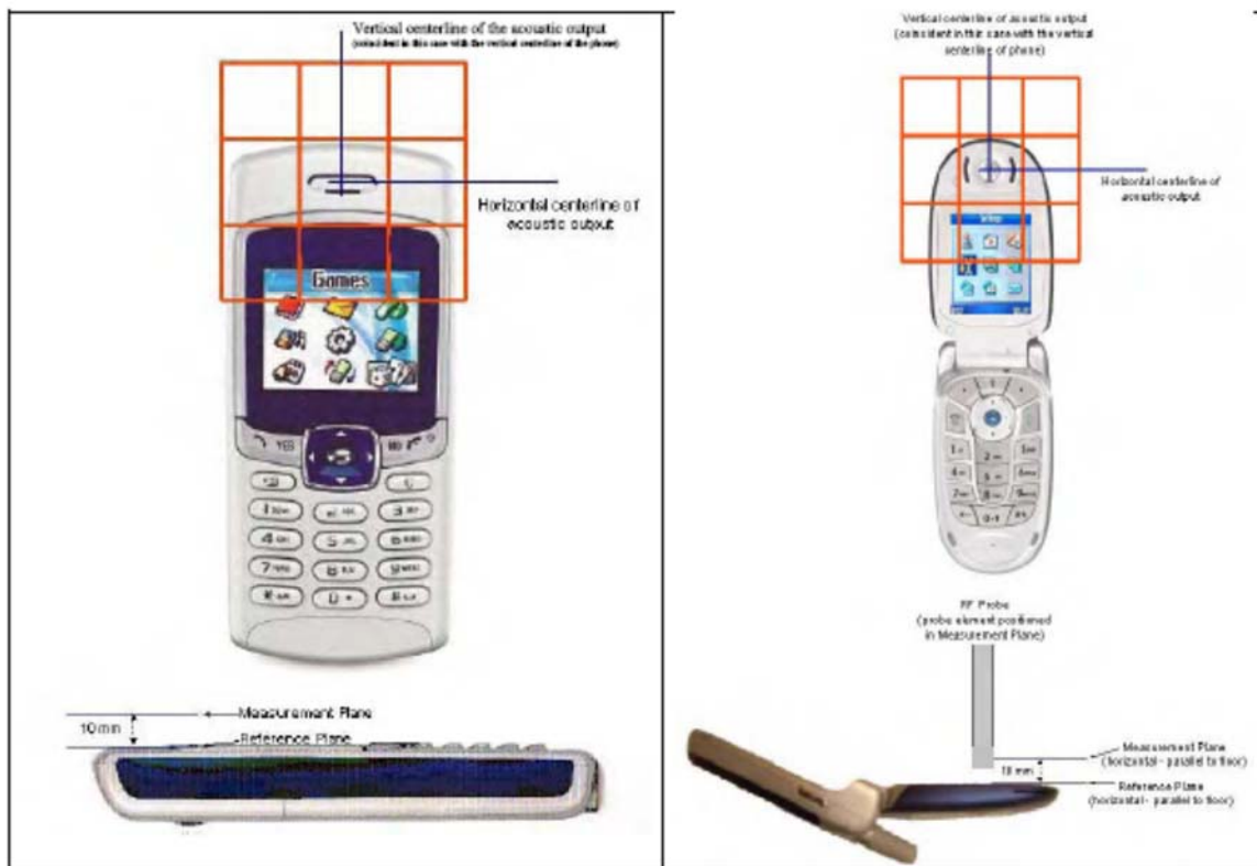
Reference and plane for RF emission measurements
