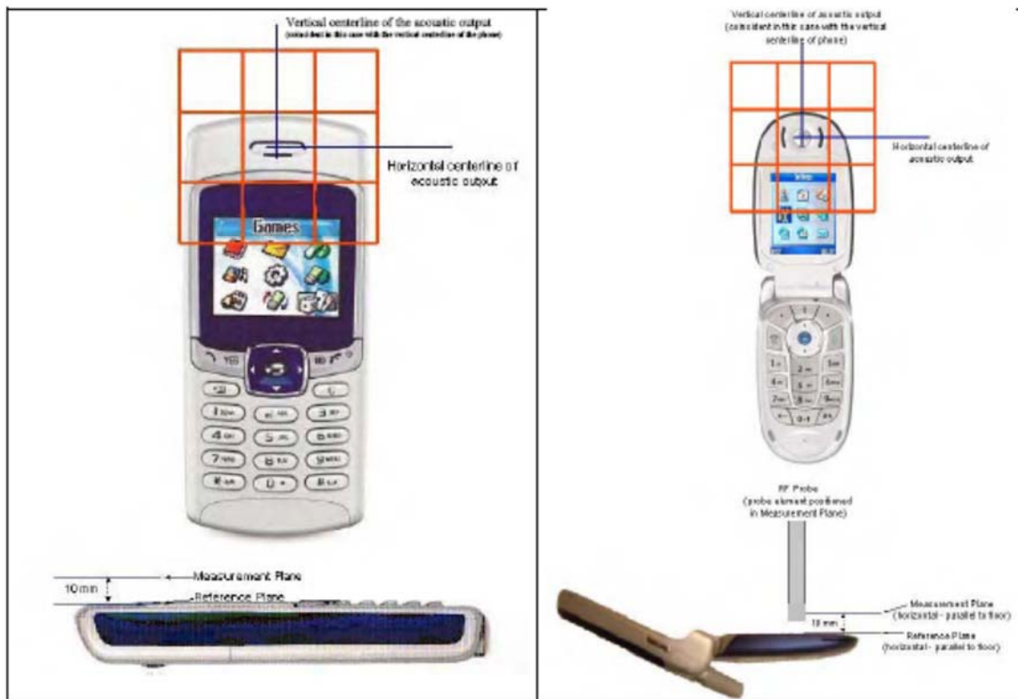
Reference and plane for RF emission measurements
