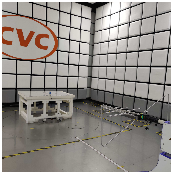
(2) Radiated spurious emission Test Setup(Above 1GHz)
