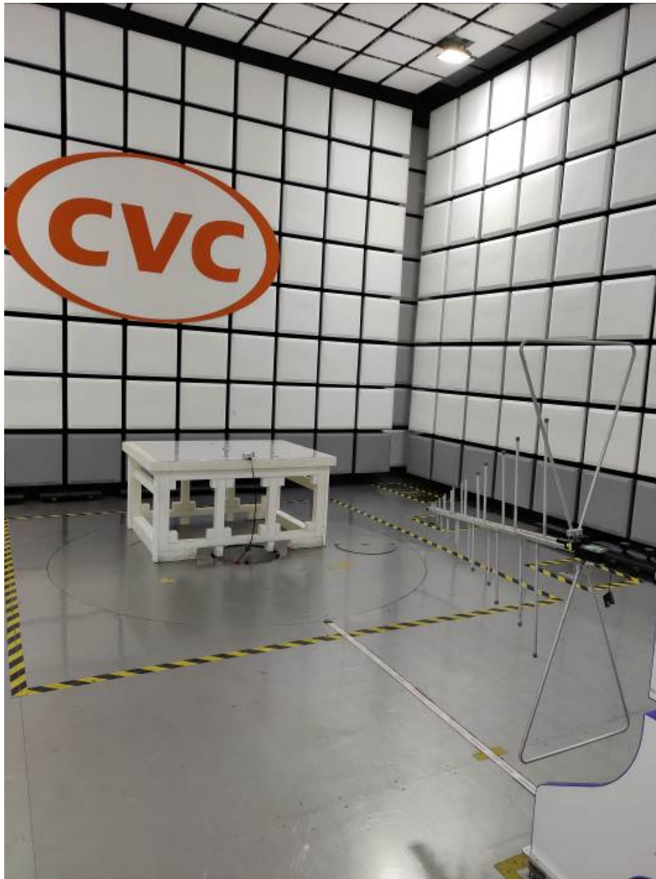
(2) Radiated spurious emission Test Setup-2(Below 1GHz)
