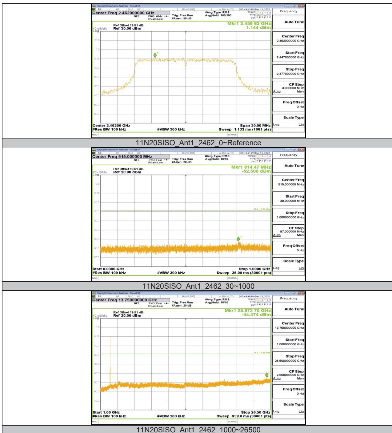
Note: The display line is placed at -20dBc but all emissions outside of the band can meet the -30dBc limit.
